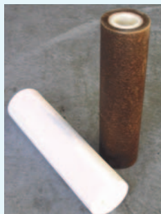
Clean and Dirty filters
